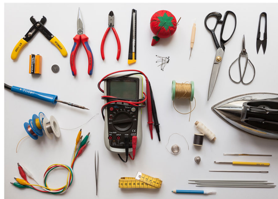
Fig. 1 Exemplary collection of tools used in e-textile making, the included tools that traditionally belong to the discipline of textiles or electronics, sometimes also to the jewelry and other related disciplines. In the center a multimeter with a pair of standard multimeter probes. A multimeter is essential to electronic measuring tasks, among others to measure resistances or detect short circuits
