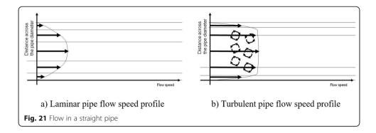
21b). In this case, there would also be a lot of eddies and vortices in the flow mixing the flow substantially as illustrated by Obeng (2012) and Fig. 1b.
